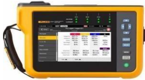
Power Quality Analyzer
